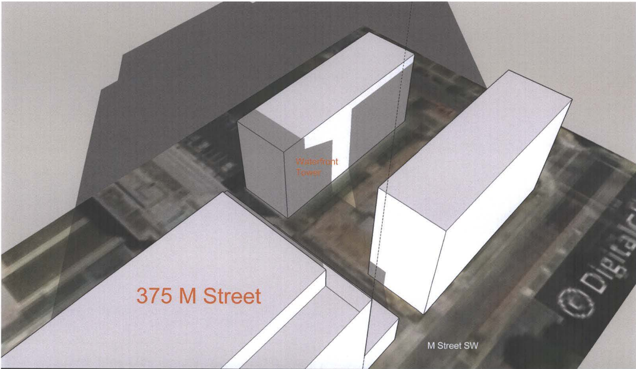
12 Story Building (375 M), 0' Setback from Alley (as proposed) 3.00pm 21 December Winter Solstice
